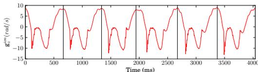
Figure 4: Segmentation of  $g_z^{ion}$  using NASC algorithm to find successive peaks, vertical lines show start times of successive segments  $(ts(n))$ .
