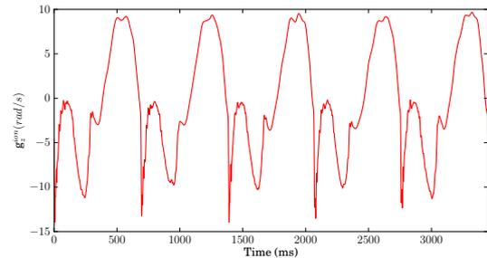
Figure 2: Example showing five steps of sagittal plane angular rate ( $g_z^{ion}$ ).
