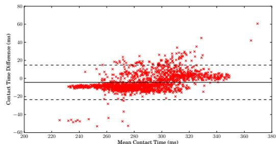
Figure 7: Bland-Altman plot of contact times derived from a heel mounted IMU.
