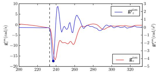
Figure 5: Heel-strike detection from sagittal plane angular rate.
